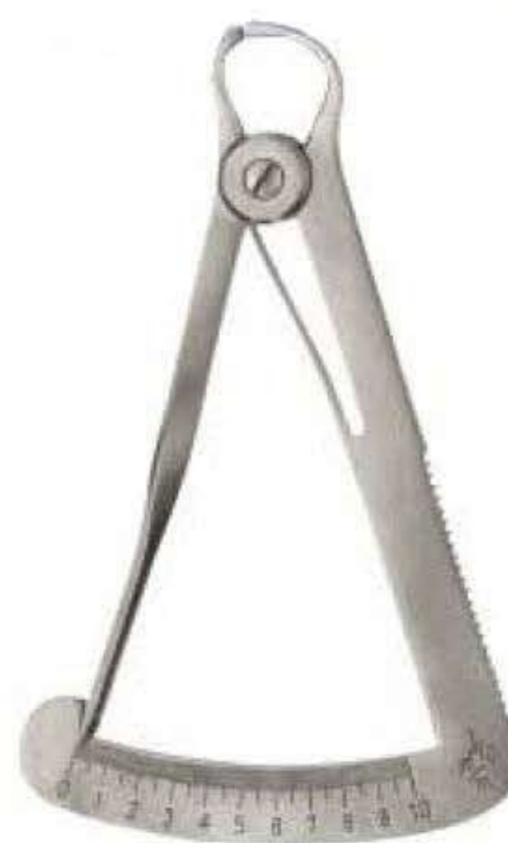
NHS-1452 Fig. 2 Iwanson spring caliper For wax.
